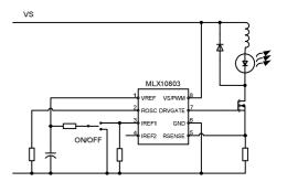
More information about how to drive LEDs and useful IC circuits can be found at: <a href="http://www.melexis.com">http://www.melexis.com</a>
