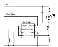
Below, one other example how in a simple way to implement slow up and down dimming effect of the LED(s).
