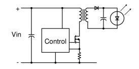
It is also possible to use the coil as a transformer in many different ways. The advantage is that you can have a very large independence with respect to the supply voltage, and high isolation between supply voltages and LED current. A bit more complicated is to also isolate the regulation feedback from the controller circuit.
