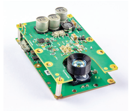
Melexis TOF evaluation kit with LUXEON IR Domed Line emitters
