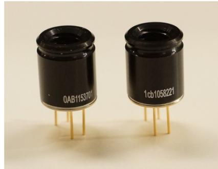
Insert the sensor in the ZIF socket on the PCB. Take care to align the notch with the silk screen on the PCB.
