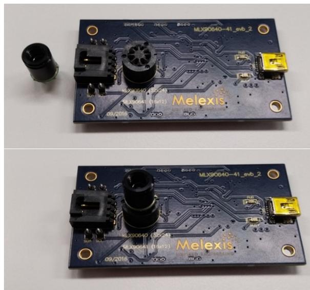
Next, connect the PCB with the USB port of the computer. The computer should indicate that a new USB device is being installed and indicate after a while it has been installed successfully. This installation normally happens only once. The pwr LED on the PCB should be on.
