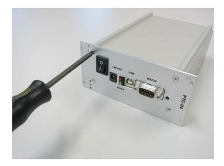
Remove the 2 bottom screws of the back panel.
