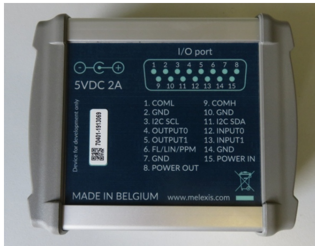
Figure 13: Pin configuration of the D-SUB15 connector
