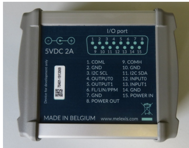
Figure 11: Pin configuration of the D-SUB15 connector
