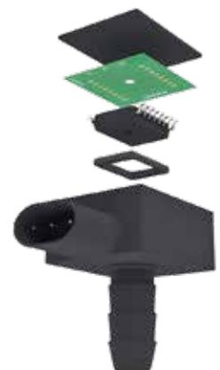
Measurement of fuel vapor pressure
