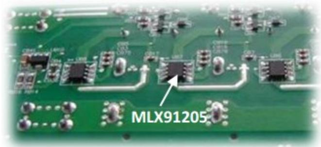
Figure 4: PDU board with MLX91205 sensors.
