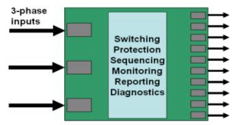
Figure 3: Simplified PDU block diagram
