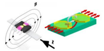
Figure 2: Current sensing principle with Triaxis™ current sensors (right) and patented IMC<sup>®</sup> technology (left)
