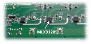
Figure 4: PDU board with MLX91205 sensors.
