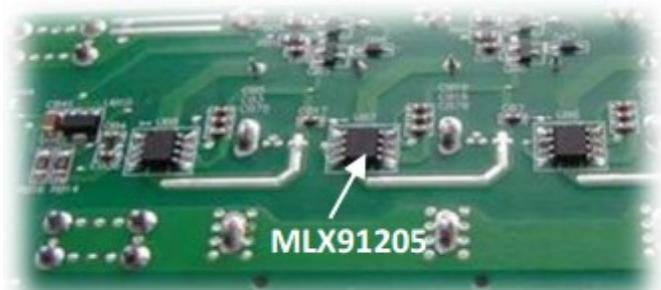
Figure 4: PDU board with MLX91205 sensors.
