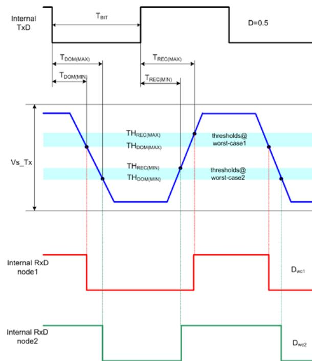
Figure 13 – LIN timing diagram, relation between propagation delay and duty cycle
