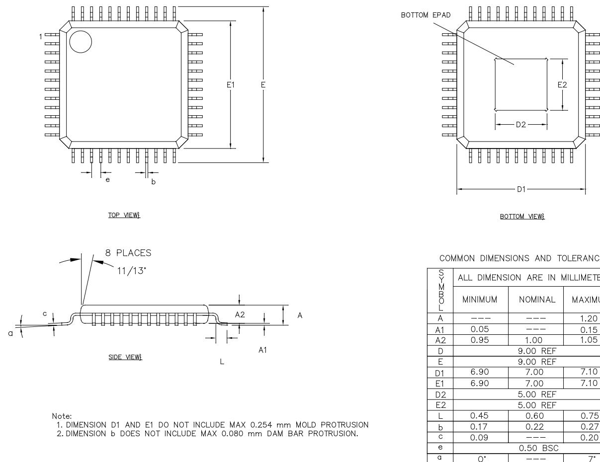
Figure 4 – Package data TQFP48 7x7 eP
