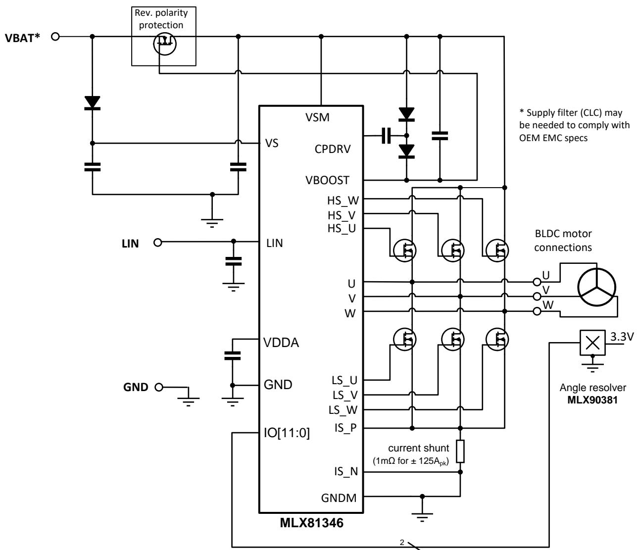
Figure 9 – Typical motor schematic with MLX81346
