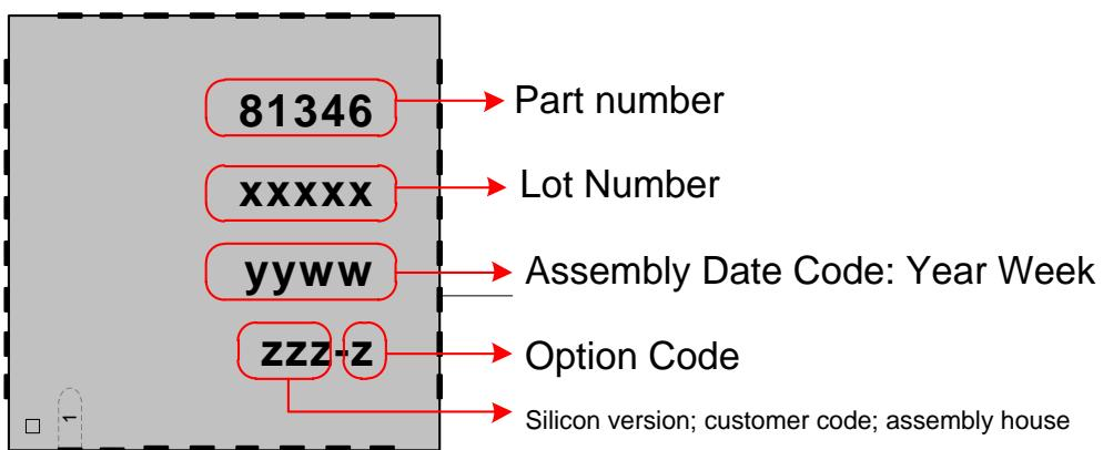
Figure 8 – Marking example on IC package TQFP48
