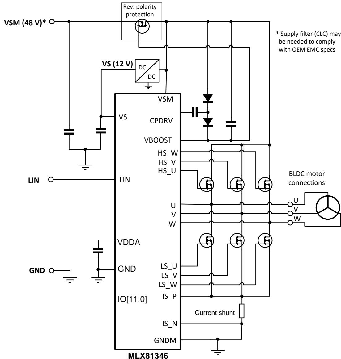
Figure 11 – Principle block diagram for MLX81346 in a 48V application
