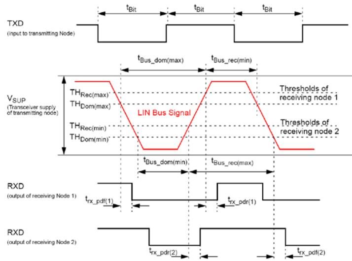
Figure 12 – LIN timing diagram (reference LIN2.1 specification)
