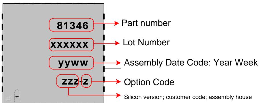
Figure 7 – Marking example on IC package QFN32 5x5
