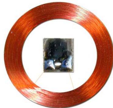
Tags were first used to identify high value items, such as cattle and horses, but are more likely nowadays to be known for their use in automotive security as either keyless entry (a chip integrated in the key transmits a code to an ECU, which opens the lock) or engine immobilizer systems.
