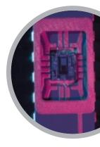
applications, Melexis Hall Devices are a reliable, contactless method of movement and position detection.
