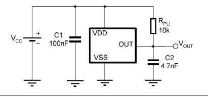
12.3. Automotive and Harsh, Noisy Environments **Three-Wire Circuit**
