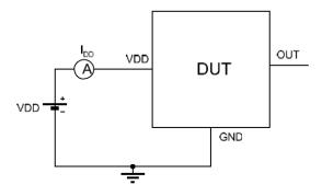
Note 1 - The supply current <sub>DD</sub> represents the static supply current. OUT is left open during measurement.
