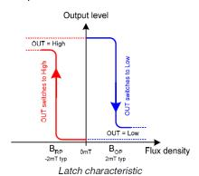
Typically, the device behaves as a latch with symmetric operating and release switching points (BOP=|BRP|). This means magnetic fields with equivalent strength and opposite direction drive the output high and low.
