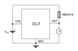
Note 1 -  $B_{\rm OP}$  is determined by putting the device under magnetic field swept from  $E_{\rm RPmin}$  up to  $B_{\rm OPmax}$  until the output is switched on.
