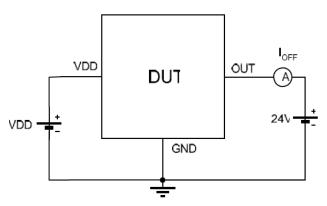
Note 1 - The device is put under magnetic field with B<B<sub>RP</sub>
