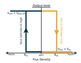
Typically, the device behaves as a latch with symmetric operating and release switching points ( $B_{OP}=|B_{RP}|$ ). This means magnetic fields with equivalent strength and opposite direction drive the output high and low.
