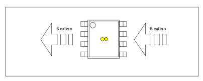
Figure 10 IMC position and geometry extra high field (XHF) version
