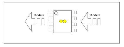
Figure 9 IMC position and geometry very high field (VHF) version
