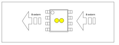
Figure 8 IMC position and geometry high field (HF) version
