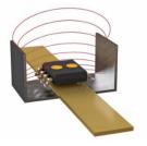
Figure 1. Typical IMC-Hall® Current Sensing Application
