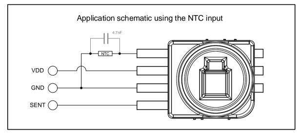
Figure 12: Basic application schematic using NTC
