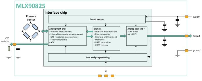
Figure 5: MLX90825 functional block diagram
