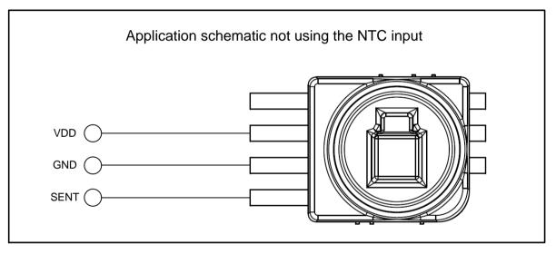
Figure 13: Basic application schematic without NTC
