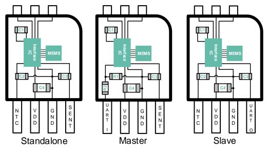
Figure 2: package diagrams of MLX90825 standalone, master and slave variants
