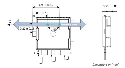
Figure 40 SMP-3 Package Sensitive Spot Position
