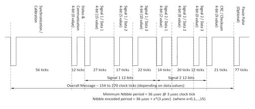
Figure 19 SENT message encoding example for two 12bits signals
