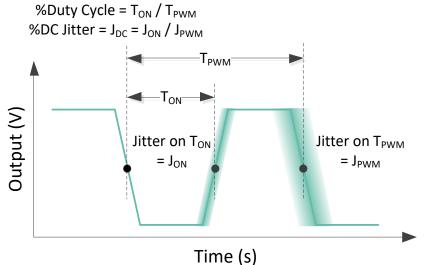
Figure 18 PWM Signal definition
