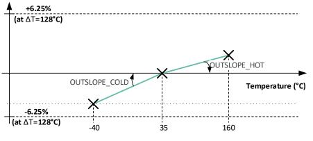
Figure 26 Temperature compensated offset
