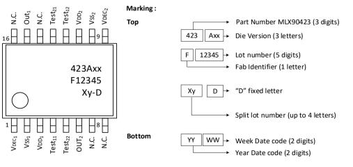
Figure 35 TSSOP-16 Package Pinout and Marking
