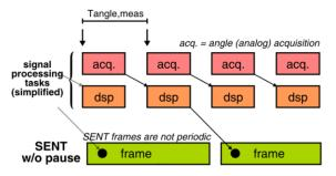
Figure 5 Continuous Asynchronous Timing Mode for SENT mode
