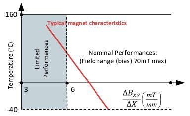
Figure 15 Minimum useful signal definition for 360° trough shaft stray field robust application
