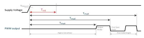
Figure 9 Startup Time Definition in PWM mode
