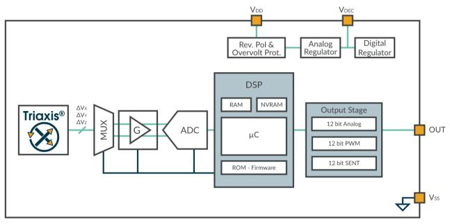
Figure 2 MLX90423 Block diagram
