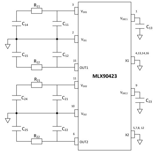
Figure 28 Recommended wiring for TSSOP-16 package (dual die)
