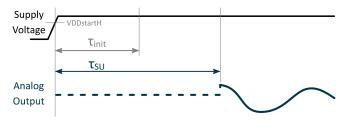
Figure 8 Startup Time Definition in Analog mode
