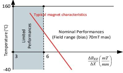
Figure 14 Minimum useful signal definition for linear stray field robust application
