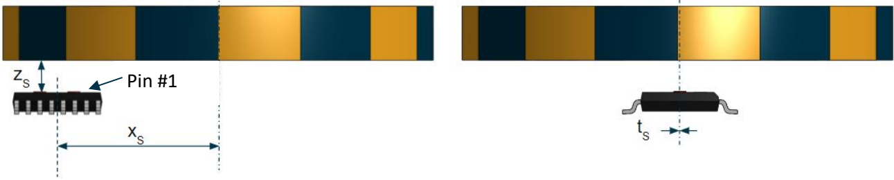
Figure 15. Assembly position of magnet and sensor chip. The chip is mounted with Pins #1 and 16 towards the ring center.
