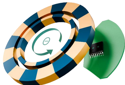
Figure 2. The Arcminaxis® Vernier sensing concept combines two sensing spots with orthogonal components
