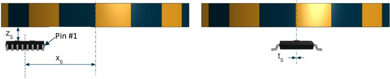
Figure 12. Assembly position of magnet and sensor chip. The chip is mounted with Pins #1 and 16 towards the ring center.
