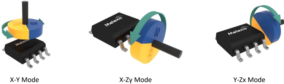
Figure 24: Exemplary illustration of the different rotary application modes
