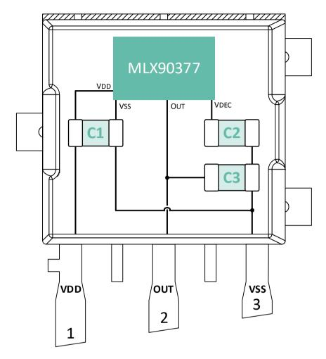
Figure 37 - Internal wiring of the MLX90377 in SMP-3
