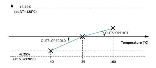
Figure 33 - Temperature compensated offset
