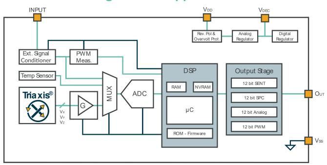
Figure 1 - MLX90377 Block diagram
