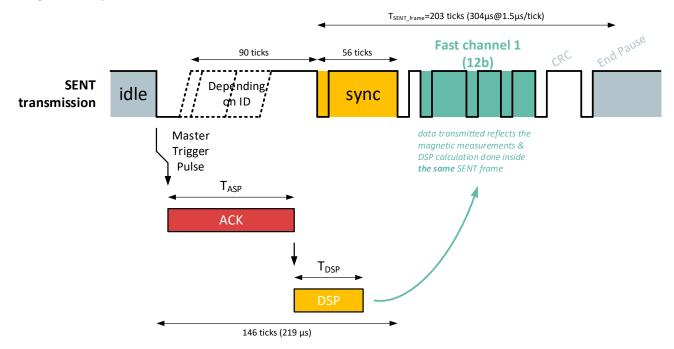
Figure 7 – SPC timing illustration in 1.5μs tick time mode and H.2 format
