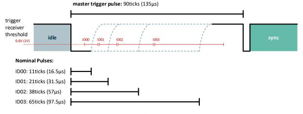
Figure 23 – Time Window for the Trigger Pulse Reception
