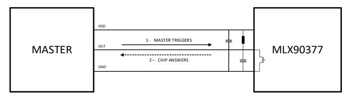
Figure 18 – SPC standard master-slave configuration
