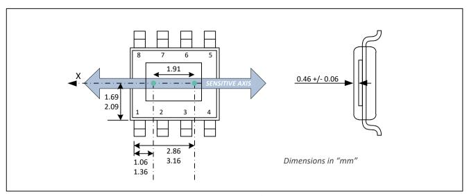
Figure 41 - SOIC-8 Sensitive Spot position for Linear Stray-Field Immune
