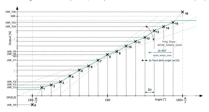
Figure 31 – 17-pts Linearization Parameters Description
