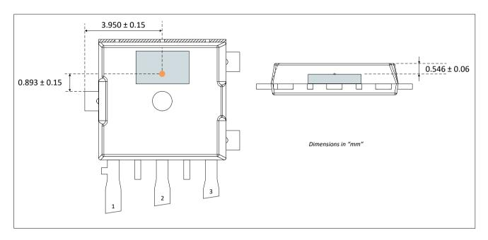
Figure 57 - SMP-3 Rotary Stray-field or legacy Sensitive Spot Position
