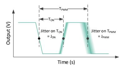
Figure 13 - PWM Signal definition
