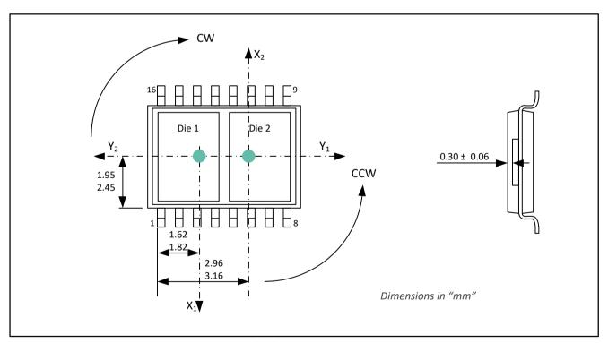
Figure 45 - TSSOP-16 dual-die package Sensitive Spot Position
