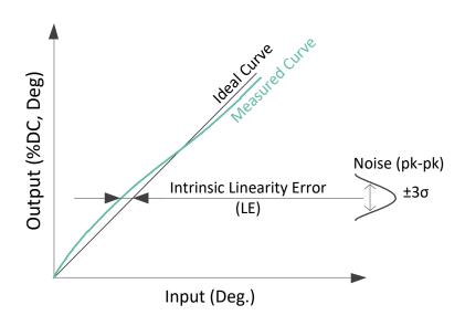
Figure 12 - Sensor accuracy definition
