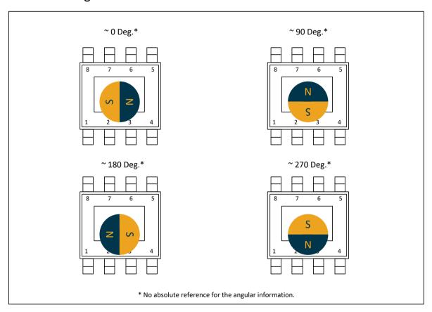
Figure 42 - SOIC-8 Angle Detection
