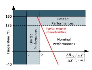
Figure 10 – Minimum useful signal definition for linear stray-field immune application
