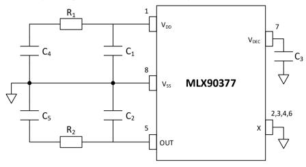
Figure 34 - Recommended wiring for the MLX90377 in SOIC-8 package
