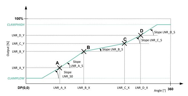
Figure 29 – 4-pts Linearization Parameters Description
