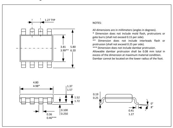
Figure 38 - SOIC-8 Package Outline Dimensions
