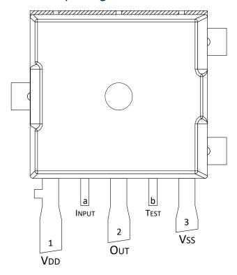
Figure 3 – Pins definition for SMP-3 Package
