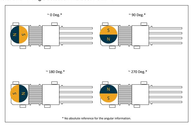
Figure 54 - DMP-4 Angle Detection
