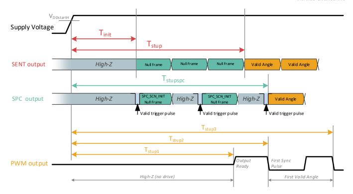
Figure 4 - Startup Time Definition
