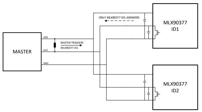
Figure 22 – SPC Bus Transmission Mode Multiplex Example
