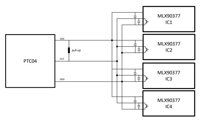
Figure 25 – Example of multiple units programming
