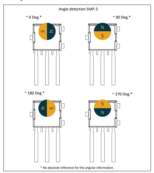
Figure 59 - SMP-3 Angle Detection
