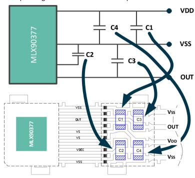
Figure 36 - Internal wiring of the MLX90377 in DMP-4
