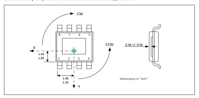
Figure 40 - SOIC-8 Sensitive Spot Position
