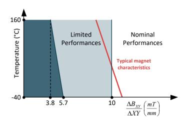
Figure 9 - Minimum useful signal definition for rotary stray-field immune application-low field variant
