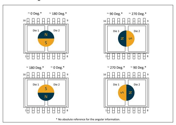
Figure 47 - TSSOP-16 Angle Detection
