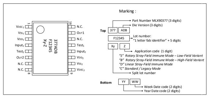
Figure 44 - TSSOP-16 Dual-Die Package Pinout and Marking
