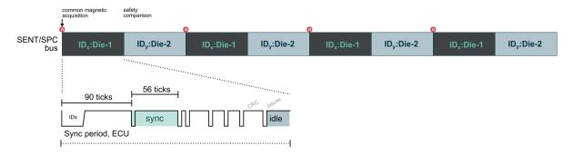
Figure 24 – Acquire Data during one SPC ID on all ICs on the same bus. Buffer and send when SPC ID matches.
