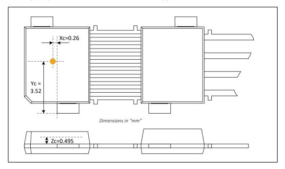
Figure 52 - DMP-4 Rotary Stray-field or legacy Sensitive Spot Position
