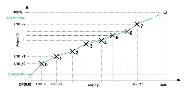
Figure 30 – 8-pts Linearization Parameters Description
