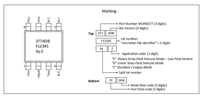
Figure 39 - SOIC-8 Pinout and Marking
