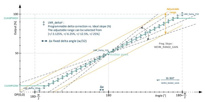
Figure 32 – 33-pts Linearization Parameters Description
