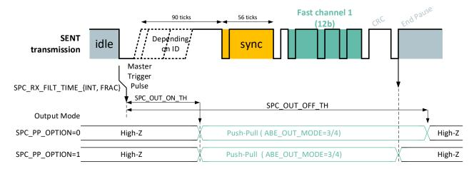
Figure 17 – SPC output driver state switching
