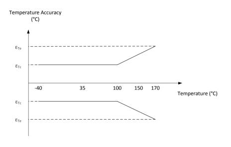
*Figure 5: NTC temperature accuracy*
