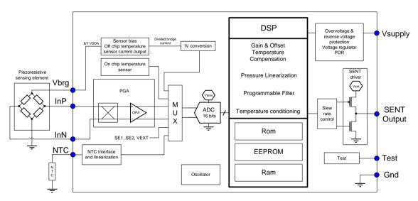
Figure 8: MLX90329 Block Diagram
