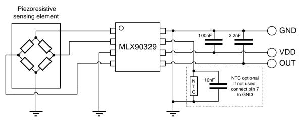
Figure 9: MLX90329 basic application schematic
