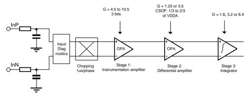
Figure 2: Analog front end block diagram
