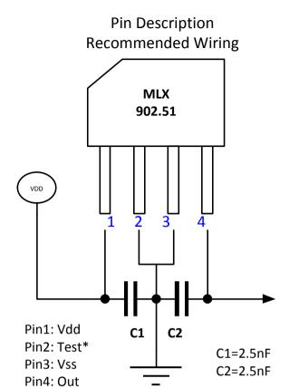
\*Readback diagnostic use only. Pin2 is not for programming device. For best results tie to Vss.
