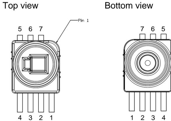
Figure 3: Package pinout
