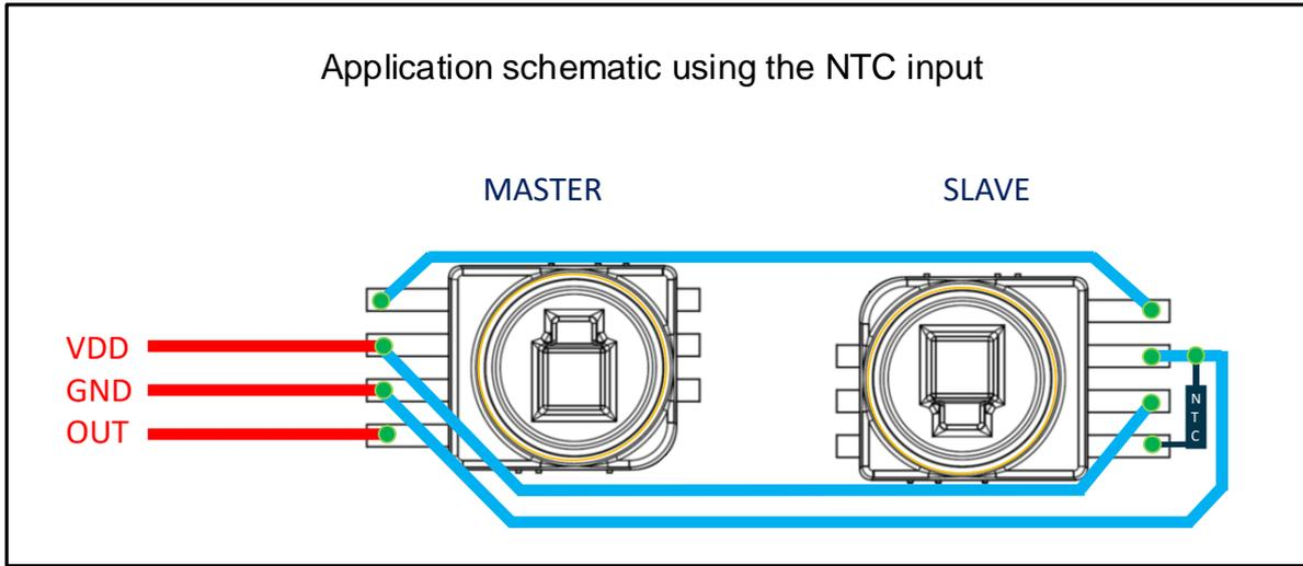
*Figure 14: Basic master and slave application schematic using NTC*
