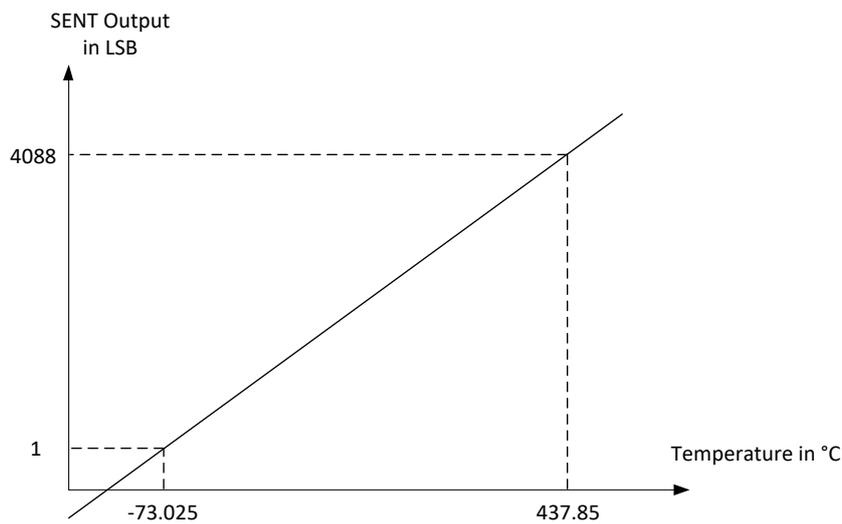
Figure 6: NTC and internal temperature transfer function
