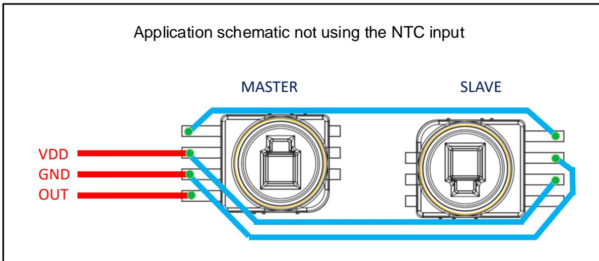
*Figure 15: Basic master and slave application schematic without NTC*
