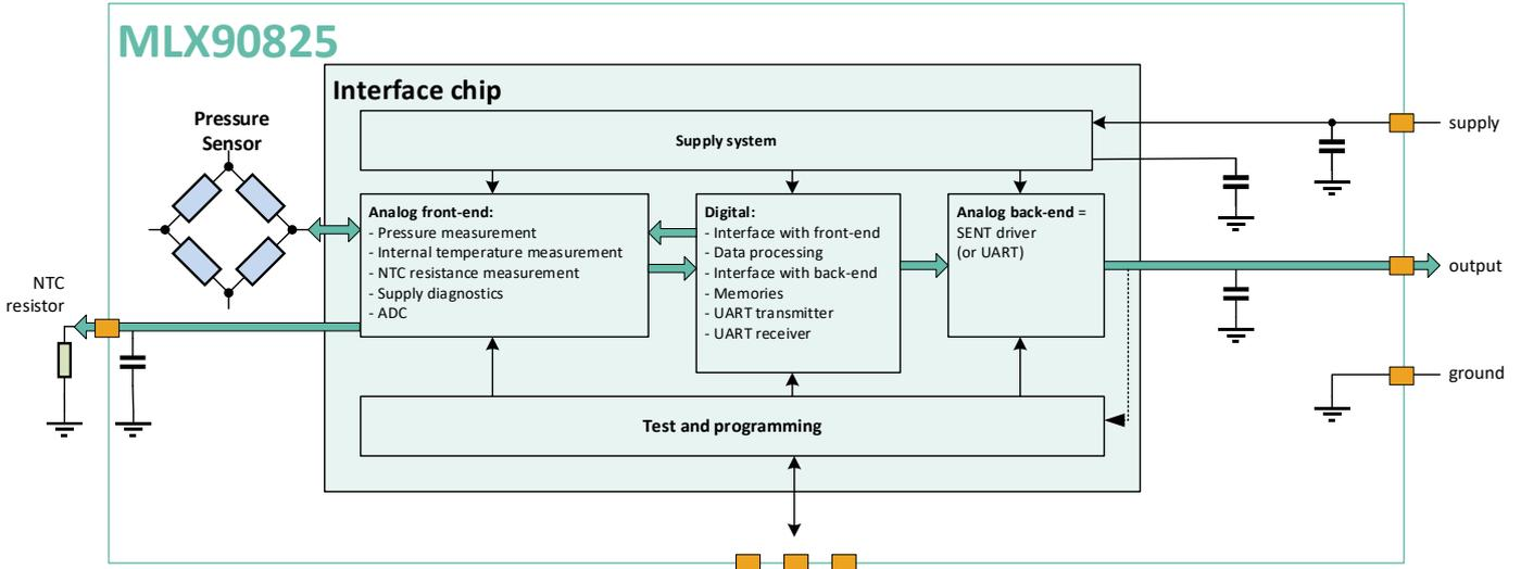
Figure 5: MLX90825 functional block diagram
