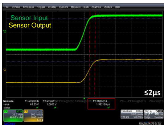
Figure 8: Sensor step response time with Noise filter OFF
