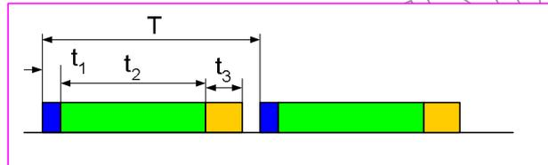
Where T is the PWM period,  $t_1$  is starting buffer (always high, with a duration which is always 12.5% of the period),  $t_2$  is the data band, taking an additional 0...50% of the period.  $t_3$  is the error signaling band (25% of the period). In normal operation the  $t_3$  should be zero as well as the rest of the period.
