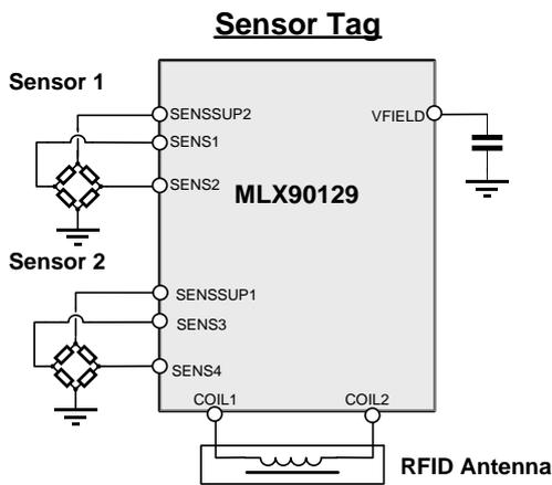
If more environmental values need to be sense, two external differential resistive sensors can be connected.
