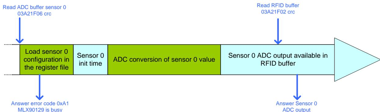
It would be exactly similar if sensor 1 configuration was used except that the setting for initialization time and for the ADC may be different.
