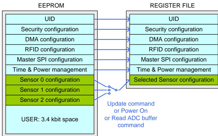
After power-on or after the RFID command “Update Register File”, the configuration of the sensor 0 in EEPROM (0x15-0x1A) is copied into the register file.
