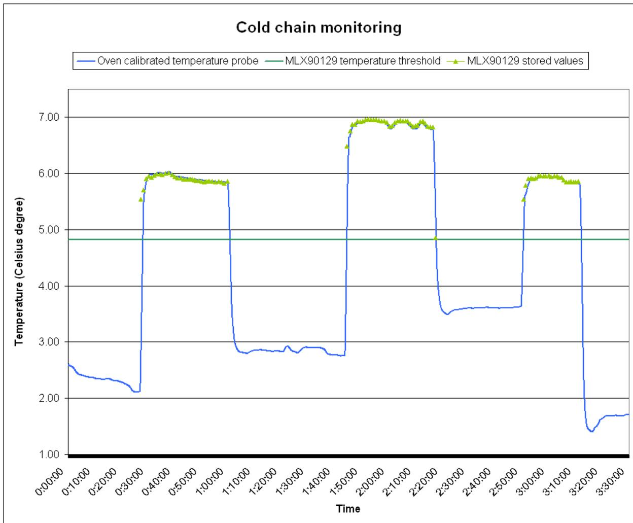
The graph shows that only temperatures above the threshold have been saved which reduces the amount of data to store.
