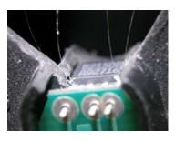
Thermocouples at B and C Experiment for temperature monitoring of pins during robot soldering
