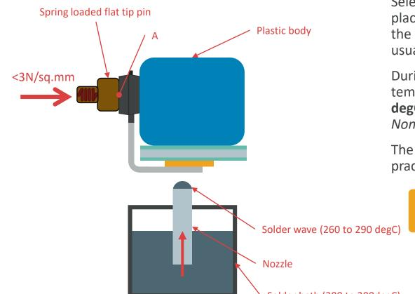
Selective wave soldering can be done with manual or automatic placement of the IC into the PCB. The solder is transported from the solder bath to the tip of the nozzle by means of a wave, usually flooded with an inert gas to avoid oxidation of the solder.
