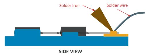
It is possible to solder PCB-less devices to fork terminals with robot point-to-point soldering.
