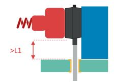
Holding pusher Flat tip to avoid mechanical damage to the mold body (UA, VA, VC, VK)
