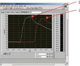
Temperature profile of A and B Differences in peak temperature are due to difference pre-heating during soldering of previous pins
