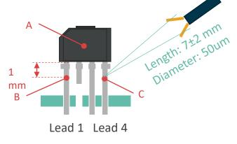
Temperature measurement positions Important points to monitor during robot soldering
