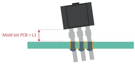
Tilting of IC due to wave soldering pushing up
