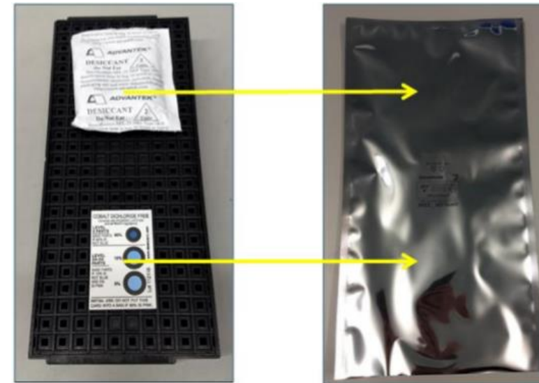
JEDEC tray with HIC and silica desiccant
