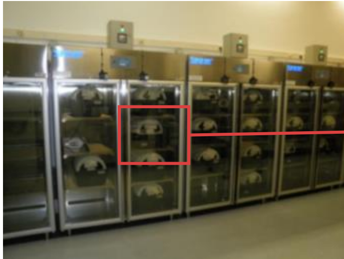
Reels on super dry oven (50C, <1% RH)
