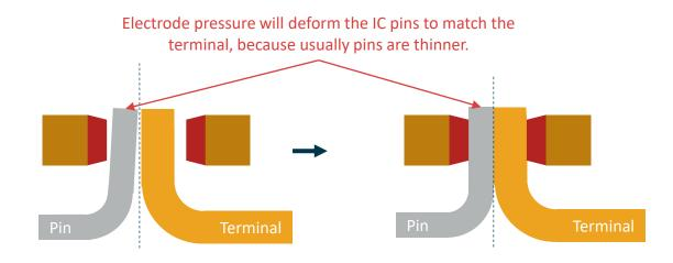
If L-shape welding is foreseen, lead forming prior welding needs to be performed on the IC, please refer to *Guidelines for lead forming of Hall* sensors in SIP package.
