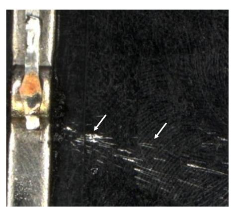
Solder ball splattering
