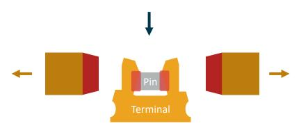
Deformation of fork and pin after welding
