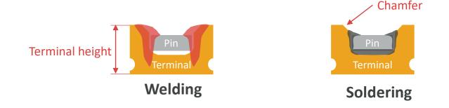
Welding to a fork terminal requires a minimum side gap between the pin and the terminal to be able to melt and forge both materials in a short time. The terminal height should be kept to a minimum, otherwise a lot of material needs to be melted before reaching the pin. It is advisable to add self-alignment features (chamfers) to the fork to help insert and align the pin to the terminal.
