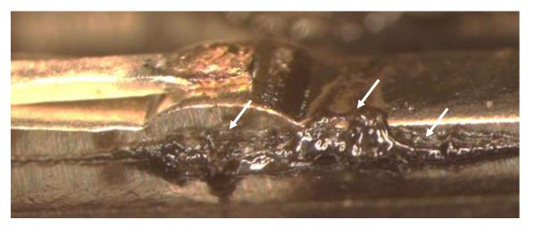
Housing plastic melting and terminal collapse
