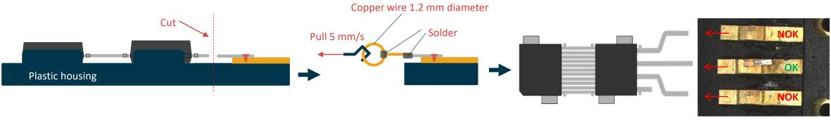
Pull test visual inspection accept/reject criteria
