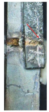
Cutting of pin with seam welding
