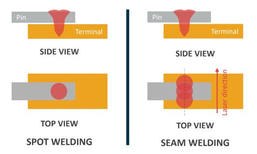
Both spot and seam welding can be used. Seam welding can be achieved by indexing the laser shots with 50% overlapping of the welds. Attention has to be taken to avoid cutting the IC lead by the laser instead of welding both metals together
