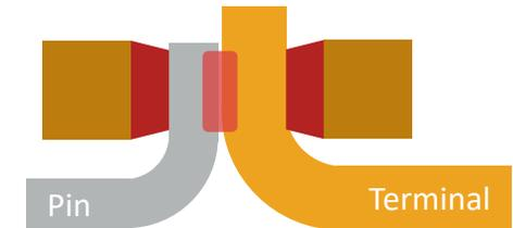
**4 – Two side electrode welding of 90 deg bent pin and terminal**
