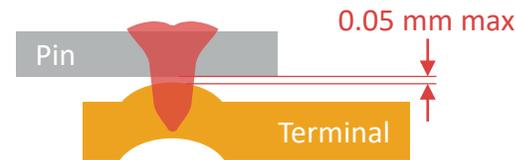
**2 – Single spot stake welding of flat pin/terminal with projection**
