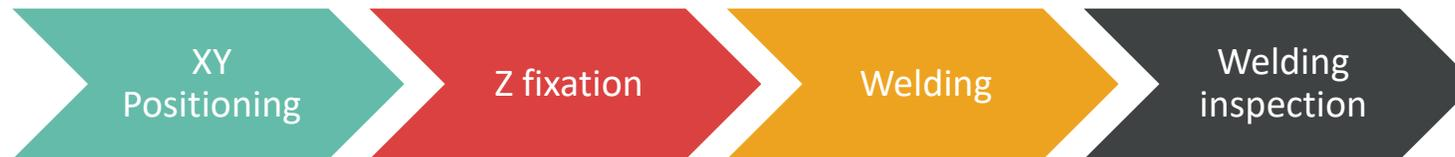
Welding of an IC to customer housing usually consists on the following steps:
