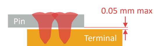
**3 – Dual spot stake welding of flat pin/terminal**
