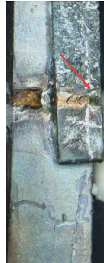
Cutting of pin with seam welding
