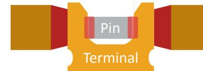
**3 – Two side electrode welding of pin in fork terminal**
