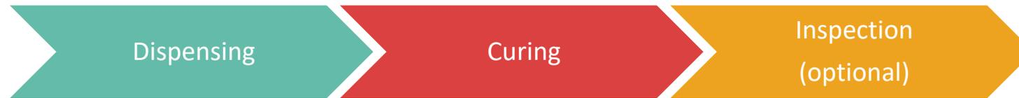
Application of potting is a frequently applied process and consists of the following steps:
