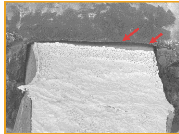
Delamination of pin from mold (exposed copper) due to insufficient clamping (SEM)
