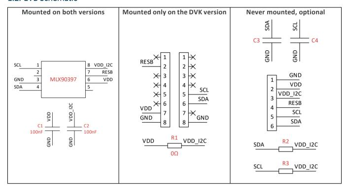
C3 and C4 are decoupling capacitors for the SDA and SCL lines, optional.
