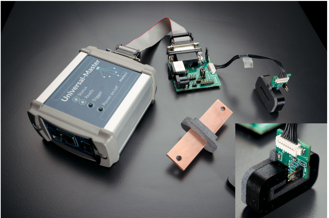
From left to right: Melexis Universal Master - Mother Board - Sensor Board (placed inside core and plastic holder assembly, zoomed view)
