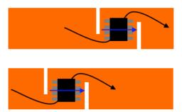
Figure 22: Current trace layout with slots and rotated sensors to avoid cross-talk between phases.
