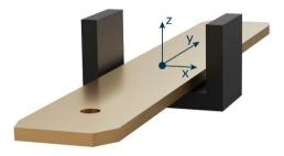
Figure 20: definition of reference system on the bus bar and shield assembly
