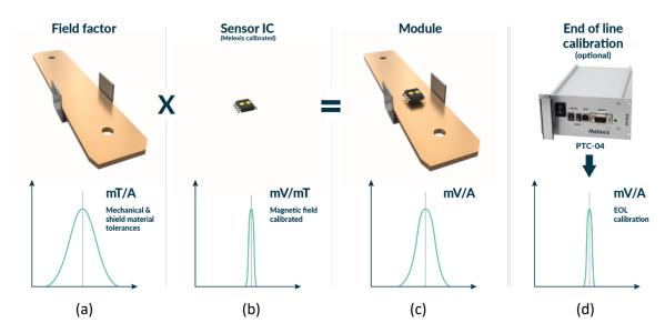
Figure 42: Sum of error of sensor and mechanical assembly. We can see that the mechanical assemble (a) introduces an error that will affect the total error (c). An end of line calibration (d) will lower again the error to the value of the sensor after fabrication (b).
