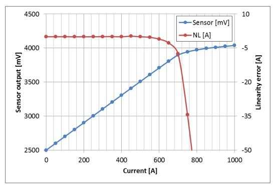
Figure 32: Sensor output and linearity error versus current.
