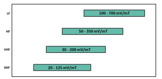
Figure 9: Sensitivity range of each IMC version.
