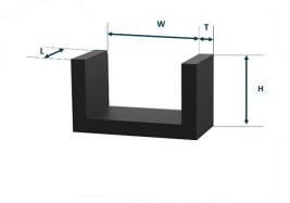
Figure 13: definition of dimensions of shields.
