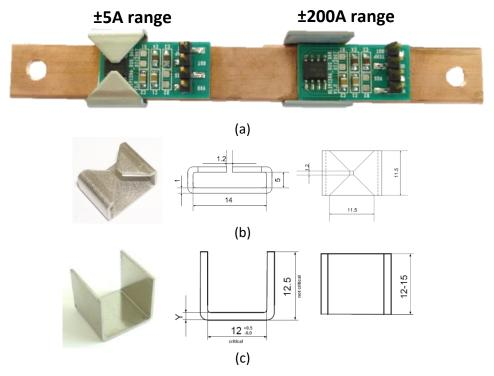
Figure 33: (a) Assembly. Images and sections for (b) closed shield and (c) U-shaped shield.
