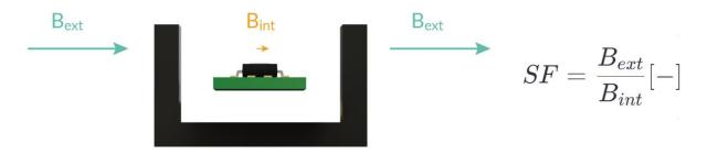
Figure 17: Shield factor definition
