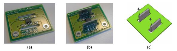
Figure 27: Single-layer evaluation board (a) without and (b) with shield. (c) Assembly instructions for shield.
