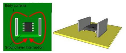
Figure 24: Current Sensing Structure – Designing the Ground Layer on the PCB such that Eddy Currents circulations is interrupted
