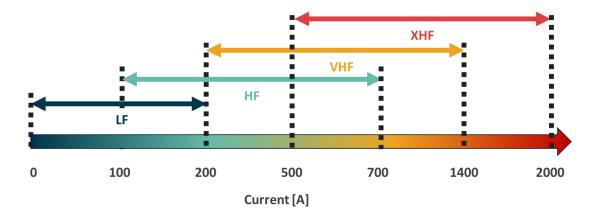
Figure 11: Optimal IMC configuration for different current ranges. Saturation of shields should also be considered. Melexis offers an online simulator tool, to choose the most optimized solution for a current sensing application, the <u>current sensor simulator</u>.
