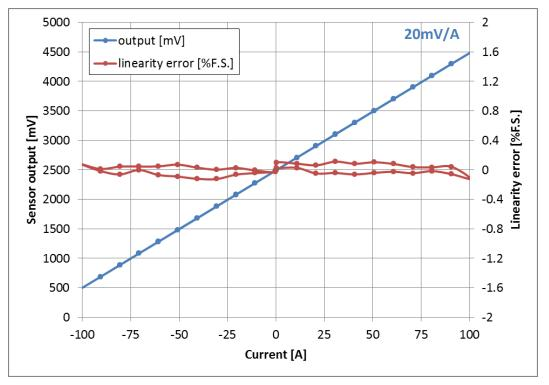
Figure 30: Typical output and non-linearity of a sensor calibrated for ±100A.
