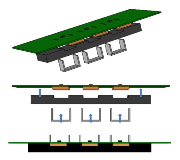
Figure 39: Assembly with pre-molded plastic case.
