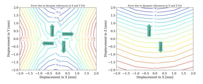
Figure 19: Effect of mechanical vibrations on the sensitivity.
