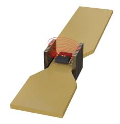
Figure 15: Necked-down bus bar example.
