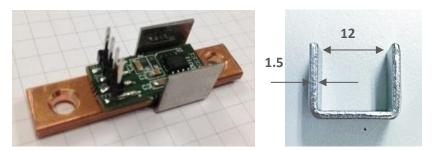
Figure 31: Demonstrator based on MLX91208 VHF sensor and U12 shield with 1.5mm thickness.
