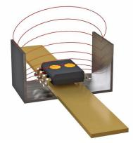
Figure 7: IMC-Hall<sup>®</sup> sensor. The yellow regions show the approximate position of the IMCs.
