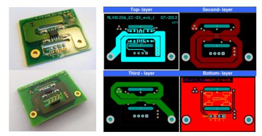
Figure 25: PCB layout example for very high sensitivity with 6 windings on 3 layers.
