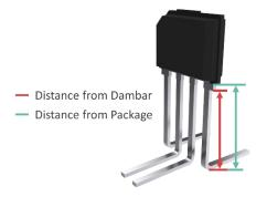
Figure 6: example of reference distances for VA package.
