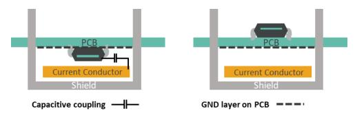
Figure 23: Current sensing structure. Expanded Ground Layer on PCB in order to reduce the parasitic coupling capacitance (coming from voltage transients).
