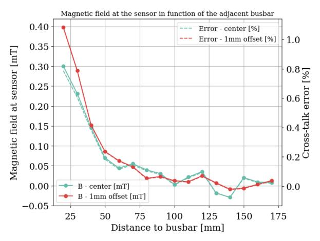
Figure 16: Cross talk error and stray field dependence with the increase of bus bar spacing.
