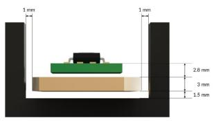
Figure 12: Shield and sensor assembly, with standard spacings.
