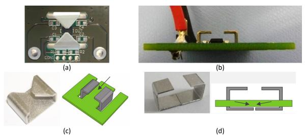
Figure 26: Top (a) and side (b) view of the full system. (c) Shield in one piece inserted through slots on the PCB edge. and (d) shield in two parts inserted in PCB slits and assembled together.
