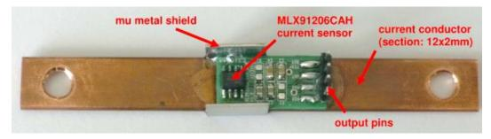
Figure 28: Demonstrator based on MLX91206 HF sensor and U12 shield with 0.8mm thickness.
