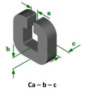
Figure 41: Ordering convention for laminated cores.
