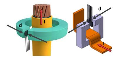
Figure 4: Example of mounting of conventional hall sensors.
