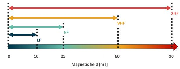
Figure 10: Linearity range for different IMC configurations.
