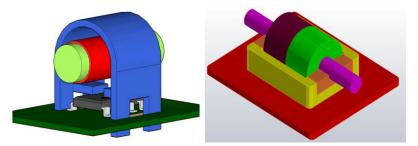
Figure 34: Cable clamp concepts (left: monolithic shield, right: two-part shield in plastic housing).
