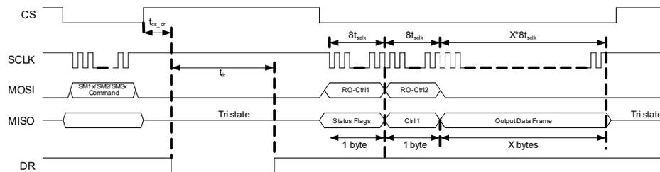
Figure 6: Timing diagram for Read-Out
