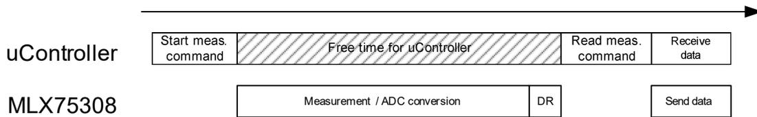
Figure 3: Measurement cycle
