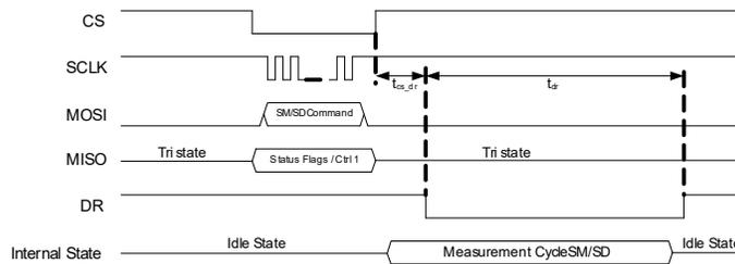
Figure 5: Timing diagram of a measurement cycle
