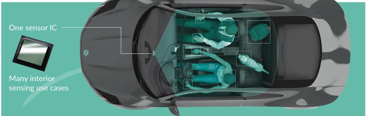
Emotion3D and Melexis have joined forces to create advanced driver monitoring system (DMS) demonstrator based on Melexis 3D ToF evaluation kit. The demonstrator shows Emotion3D's attention-monitoring technology using Melexis automotive qualified 3D ToF sensors. It enables robust head tracking, eye gaze and eye closure for in-cabin driver monitoring.
